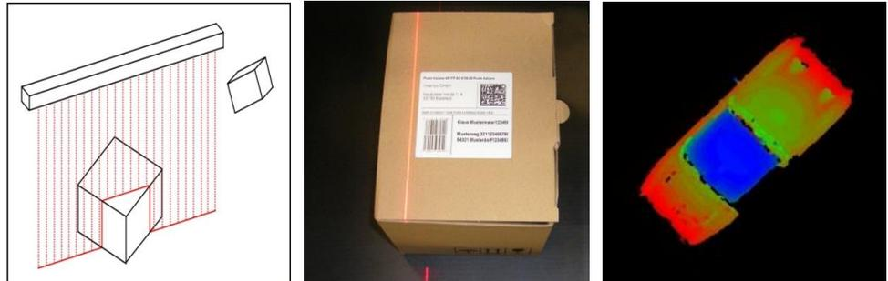
The laser scanning technique is a light striping technique which is used for 3D measurements of object surfaces. To acquire the 3D information, the object is moved relative to a laser line, while it is observed by a camera. The camera must be positioned outside the laser plane. Due to the different heights of the object, the camera will see a shifted laser line according to the height of the object. From this shifted laser line, the height of the object can be back-calculated.
